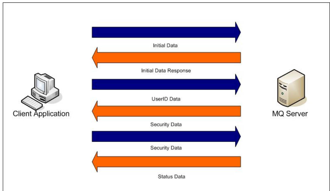
Figure 16 - an overview of the packets exchanged during authentication with a Security Exit
